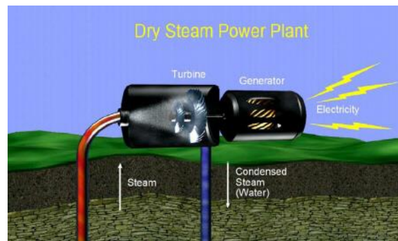
Figure 6. Dry steam power plant.
