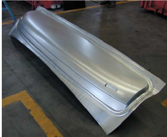
Figure 9. Front panel of a car body before trimming operation
