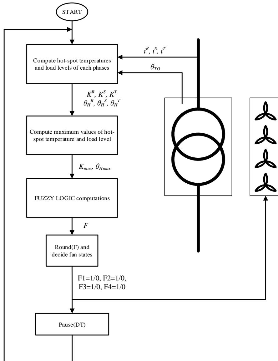
Figure 4. Structure of the proposed transformer cooling control
