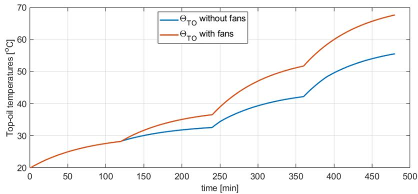
Figure 7. Top-oil temperatures in cases with and without fan
