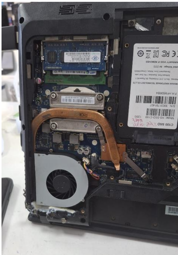
Figure 2. The photograph of the connection of the heat pipe on the laptop.
