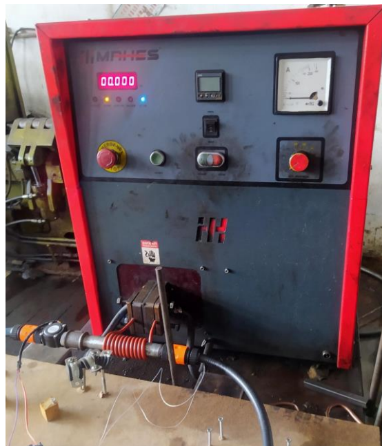
Figure 2. Figure 2. Induction heating machine (380 Volt, 25 kW).
