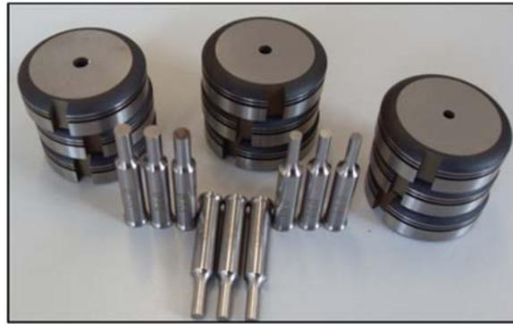
Figure 1. AISI D3 tool steel punch and die (5, 6 and 7 mm).
