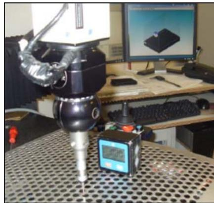
Figure 8. The measurement setup in the CMM.
