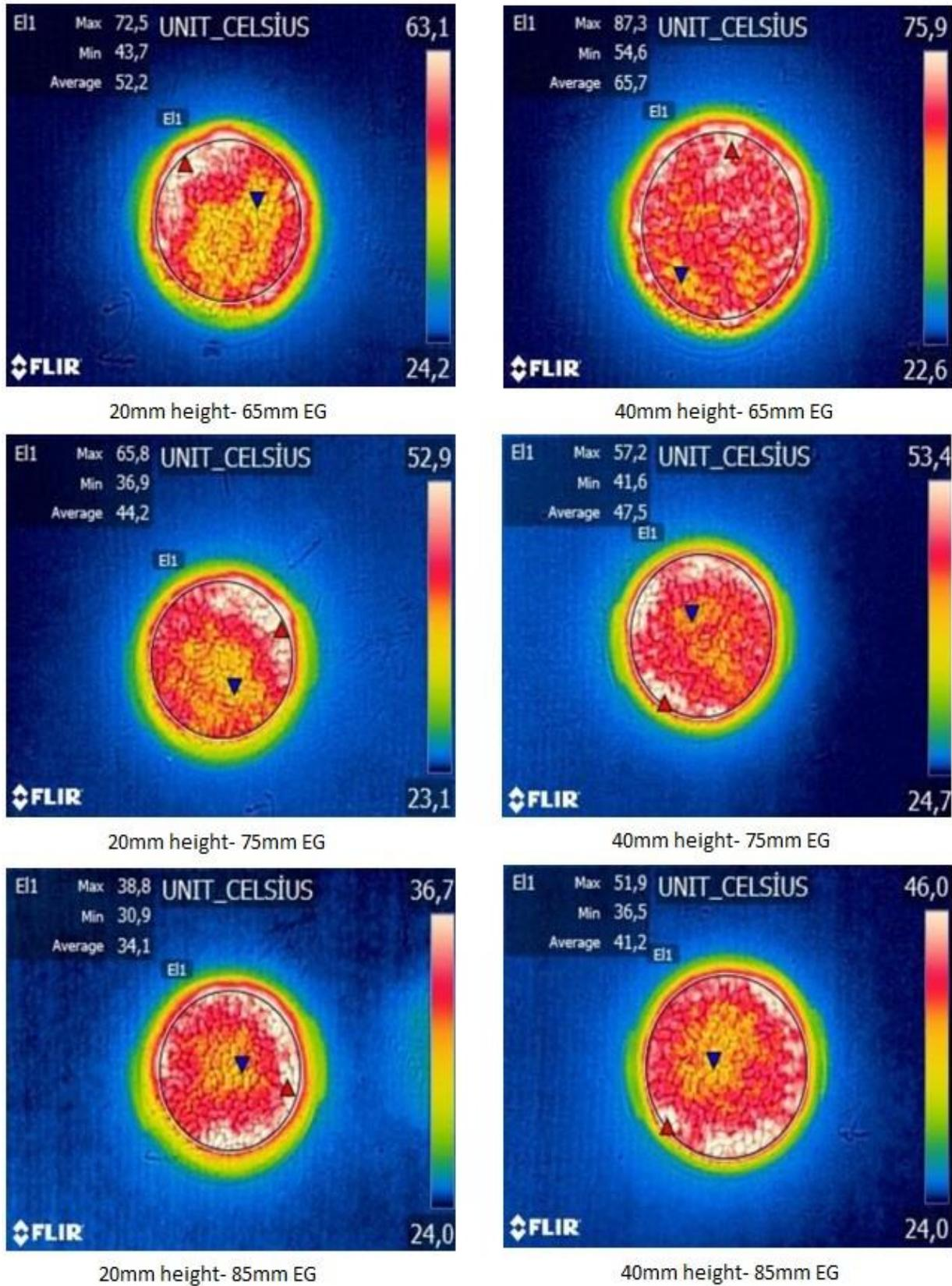
Figure 5. Thermal images of the specimens for three EG and two heights bean specimens.
