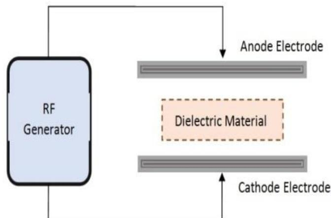
Figure 1. The schematic diagram of parallel plate RF heating system.
