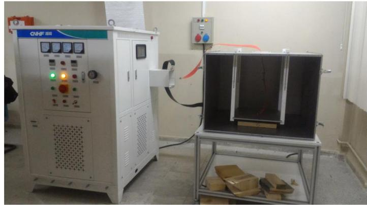
Figure 2. RF generator and integrated oven.
