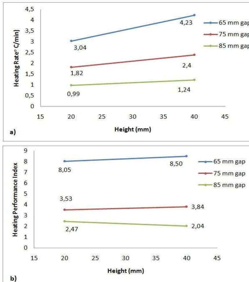
Figure 3. a) HPI and b) HR change depending on electrode gap.
