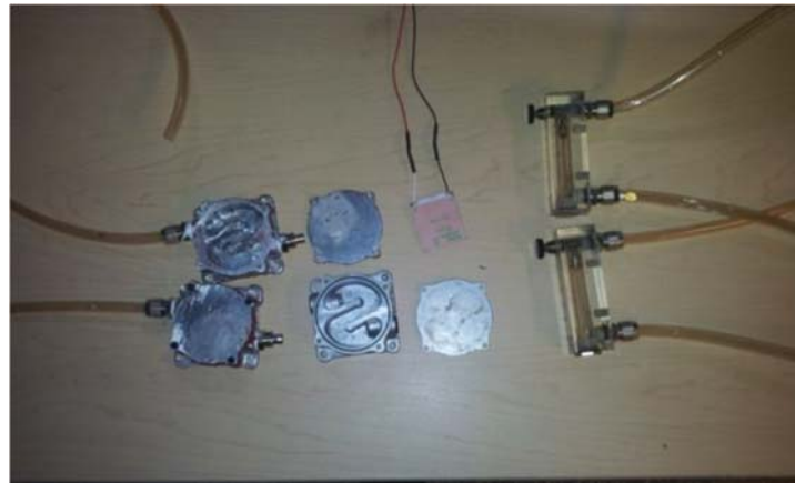
Figure 4. The individual parts of the peltier system with tubed rotameters.
