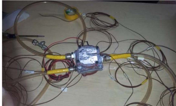
Figure 3. The peltier unit with thermocouplers planted.
