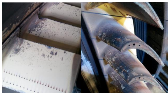
Figure 9. Melted blades under bad cooling condition.
