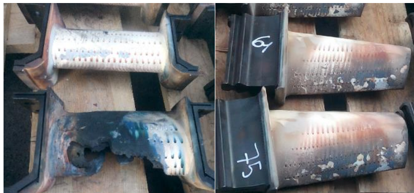
Figure 11. Melted blade and vanes.
