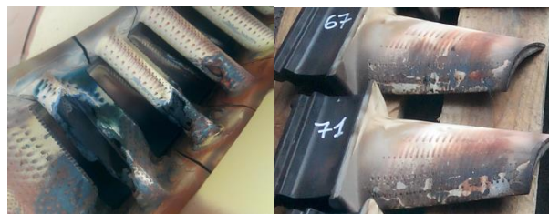
figure 7. Melted blades under bad cooling condition.
