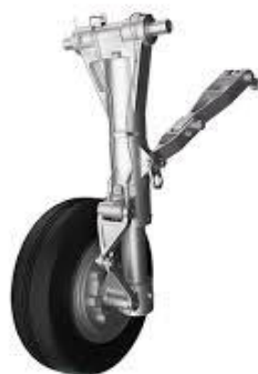
Figure 4. Image showing the landing gear of an aircraft [8]
